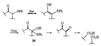
A reasonable rationale mimics the two-step process reported in the first part of this paper. Thus, hydroxylation of the enol form of the  $\beta$ -keto sulfide in a slow step ultimately to generate the diketone is analogous to the facile acetoxylation with lead
