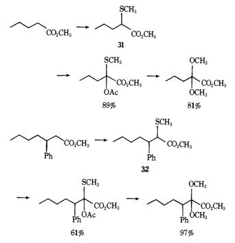
erably slower and required 35-45 h for completion. The slower rate may be attributed to the lower acidity of these sulfenylated derivatives compared to the  $\beta$ -keto sulfides. Nevertheless, the reactions were clean and good yields were obtained. Conversion to the methyl ketals proceeded smoothly as before.
